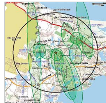
Vaisala STRIKEnet® online analysis uses NLDN historic data to pinpoint lightning activity relative to suspected lightning damage.
