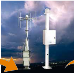
Sensors instantly detect the electromagnetic signals created when lightning strikes the earth's surface.
