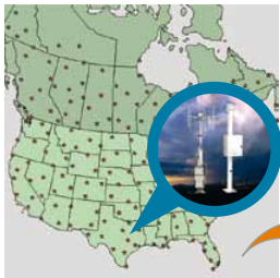
U.S. NLDN consists of more than 114 remote, ground-based lightning sensors.
